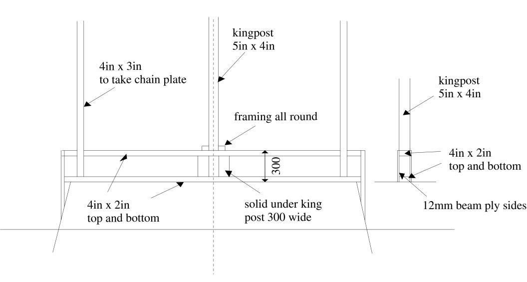
Revised Flica mast beam other details on Building Plan sheet
